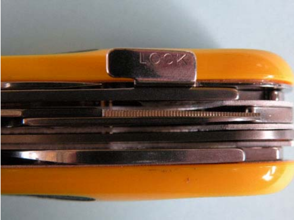
EvoGrip S18 main blade locking mechanism
